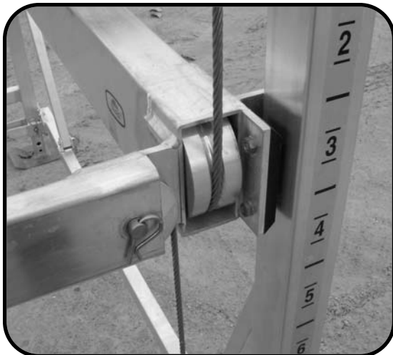
ALUMINUM SHEAVES - STAINLESS PINS WITH GREASE ZERKS - STAINLESS CABLES. GREASE PINS WITH ZERKS YEARLY
