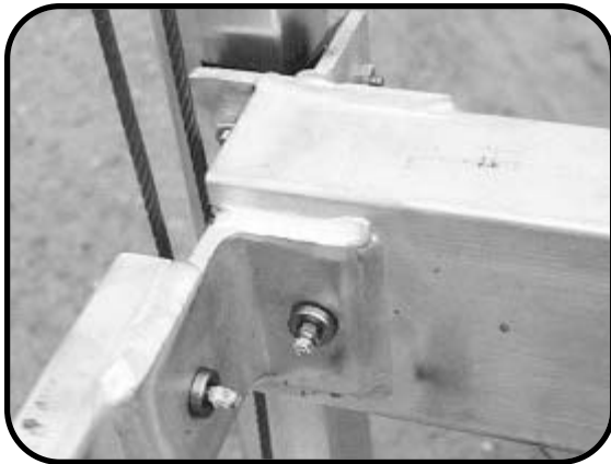
ALUMINUM SHEAVES - STAINLESS PINS WITH GREASE ZERKS - STAINLESS CABLES. GREASE PINS WITH ZERKS YEARLY
