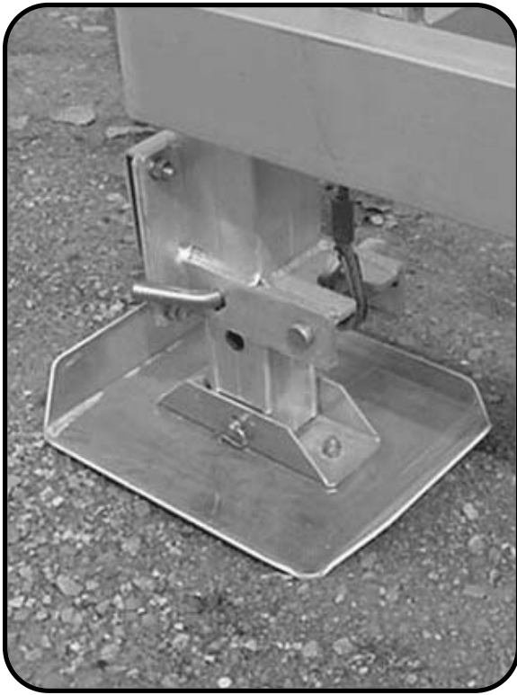
EYE END OF CABLE. INSERT PIN THROUGH FLATE AND EYE. INSTALL HAIR PIN.
