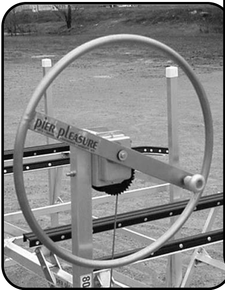
D.L. WINCH AND WINCH WHEEL INSTALLED. SECURE WHEEL BY ATTACHING WINCH WHEEL WASHER WITH SPACER AND BOLT SUPPLIED WITH D.L. WINCH KIT.
