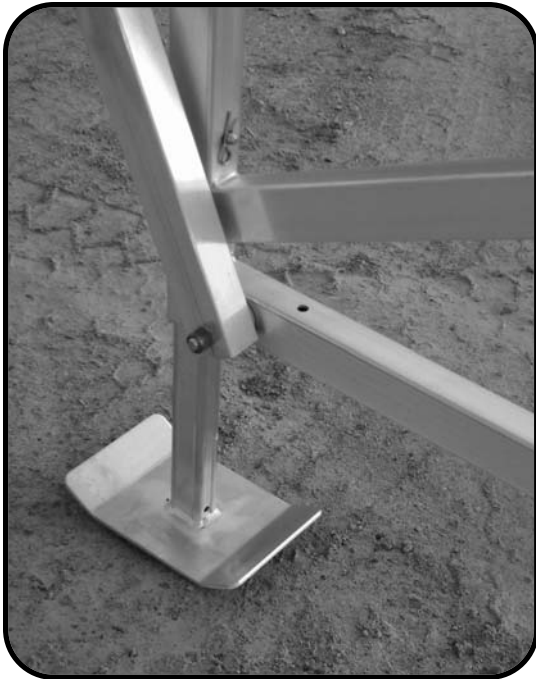
REAR CANTILEVER ATTACHED TO LEFT SIDE USING 1/2" x 4" BOLT, PLASTIC WASHER IN BETWEEN, AND BRASS NYLON LOCK NUT.
