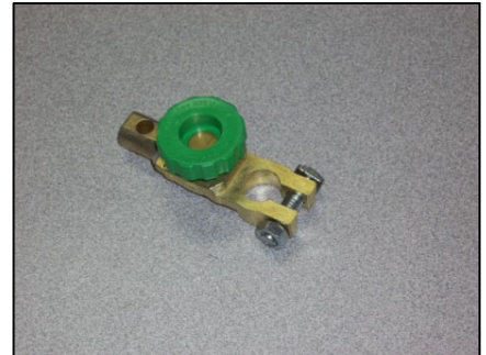
System Shut-Off Switch
