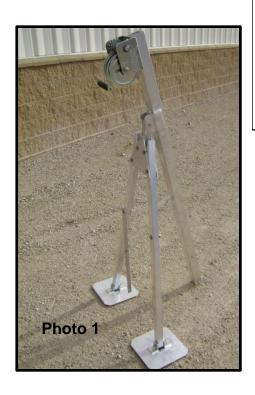
All bolts must be installed and securely tightened before using the tripod winch. Failure to have all bolts in place could result in damage to the dock or serious bodily injury.
